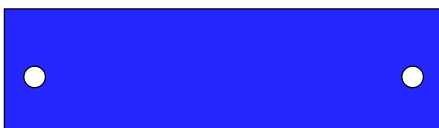
20mmx200mmx5mm Flat bar to brace segments together
